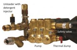
ASP (Aussie Safety Protection) kits, include thermal dump valve & safety valve. Protects operator & machine against excessive bypass & pressure spikes.
