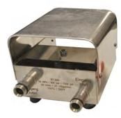
Stainless steel housing, & valve, rubber feet, includes 3m whip hose max 500 bar, 40 lpm, 150°C M24 M Inlet Outlet M24 M
