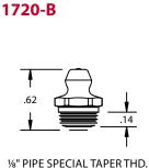
%" PIPE SPECIAL TAPER THD. (Recommended hole size-.373 to .380")
